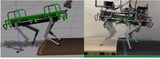
Fig. 6. HyQ robot stepping up a pallet of 10cm in both simulation (Gazebo) and hardware experiment.
