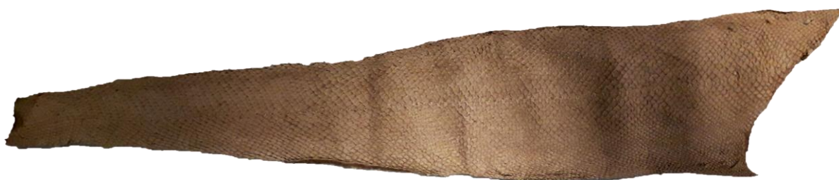
Figure 24. Photo of salmon fish leather obtained by mimosa and chromium tanning.
