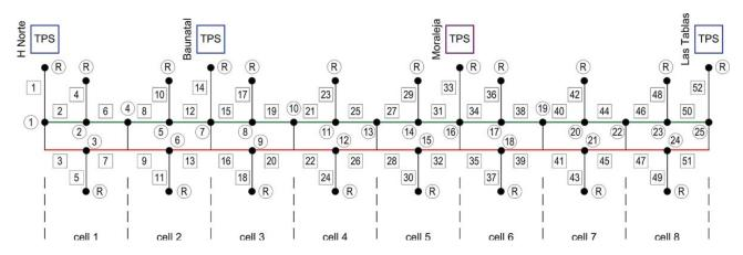
Fig. (2). Line diagram with branches (numbers in square frame) and nodes (numbers in round frame); the two lines are distinguished by green and red color. The topology refers to line 10 of Metro de Madrid, where the Moraleja TPS is really a bidirectional substation after the upgrade of few years ago.
