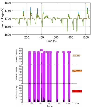
**Fig. (3). a)** Profiles of pantograph voltage for different scenarios of nominal values (all related to 1700 V by applying an offset for graphical purposes): 1600 V blue ("Mor1"), 1650 V orange ("Mor2"), 1700 V brown ("Mor3") all with a 1680-1800V pair of min-max threshold value for the operation of the onboard rheostatic chopper. **b)** comparison among the braking rheostat current behavior for the three cases.
