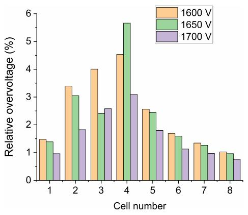
Fig. (6). Profiles of relative overvoltage, for different substation voltage supplies  $V_{ESS}$ , produced by the regenerative braking for the case of two reversible substations placed in H-Norte (cell 1) and Las Tablas (cell 8) stations.
