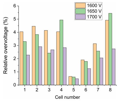
Fig. (5). Profiles of relative overvoltage, for different substation voltage supplies  $V_{ESS}$ , produced by the regenerative braking for the case of one reversible substation, La Moraleja, placed between cell 5 and cell 6.
