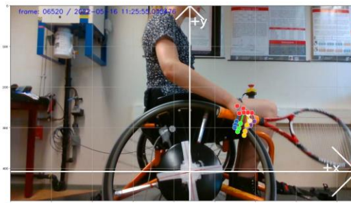
Figure 2: RGB image acquired by the camera placed on the right with hand landmarks detected by Mediapipe. The origin of the reference frame is placed in the centre of the wheel
