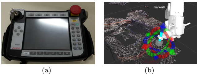
Fig. 3 (a) The teaching pendant for an industrial robot from Denso Corporation. Each joint of the robot can be controlled using two rows of buttons, at left. (b) A 6-DOF 3D interactive marker in the robot operating system (ROS) that can be manipulated with a mouse by pulling arrows for translation or dialing rings for orientation control.
