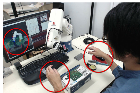
(c) Trying to set up the orientation of the end effector with hand gestures.
