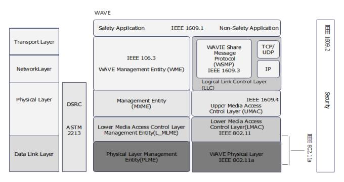
Figure 2: WAVE, IEEE-1609, IEEE-802.11p With Network Layers.
