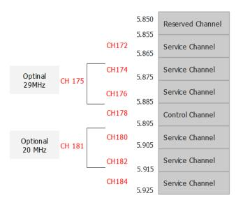
Figure 1: DSRC communication channel
