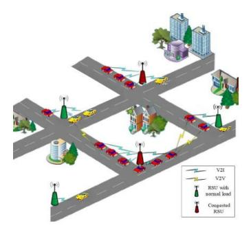
Figure 3: VANET Network (V2V, V2I)
