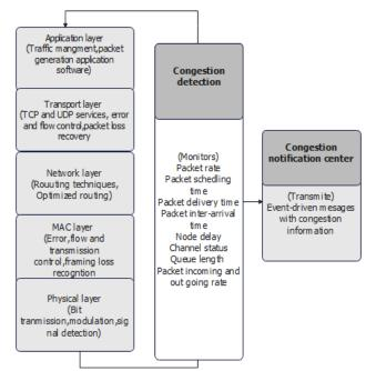
**Figure** 5: Cross-layer Procedure in Congestion Detection model.
