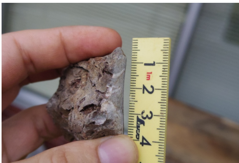
Photo 6. Quartz-Calcite vein partially removed. The picture shows a rock fragment from the borehole core sample.
