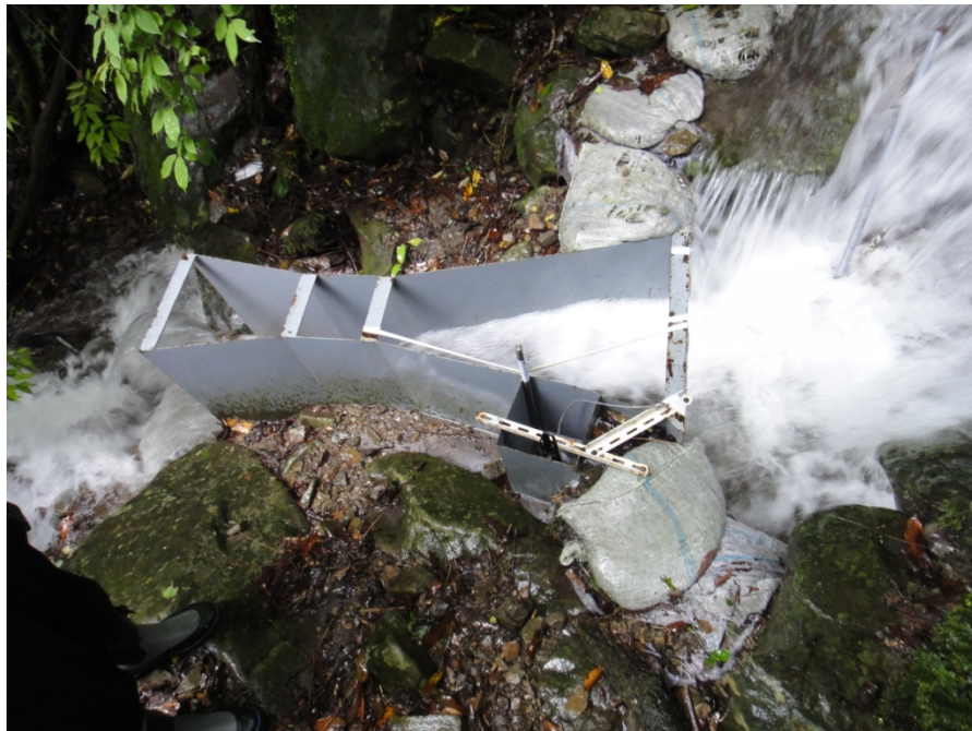
Photo 12. Parshall flume in catchment U.
