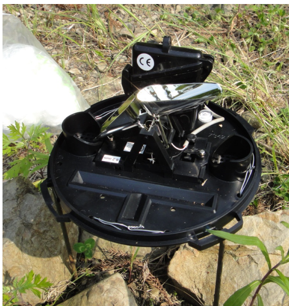
Photo 14. Open tipping bucket rainfall gauge.
