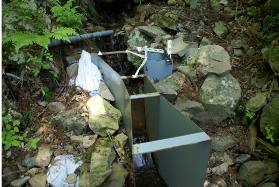
Photo 11. Parshall Flume in catchment D.
