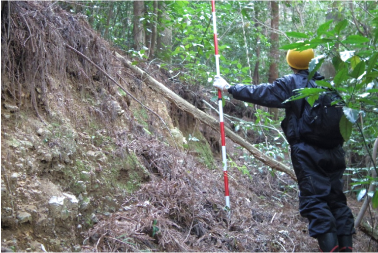
Photo 7. Gravitational deformation scarp near to the ridge in the studied hillslope.
