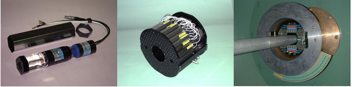
Figure 3.4: (Left)An element of the BBC composed of a mesh-dynode photomultiplier with a quartz radiator. (Middle)A BBC composed of 64 elements. (Right)The BBC installed around the beam pipe behind the Central Magnet.
