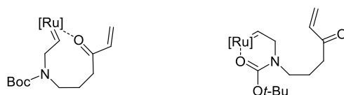
Figure 13: Complexation of the ruthenium-carbene intermediate could hamper ring-closing metathesis. Addition of Ti(Oi-Pr)_4 as Lewis acid can prevent this complexation. 7,12,13
