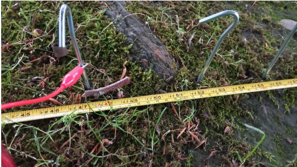
Figure 51. Depiction of the survey. Stainless steel pegs were used as electrodes and the root was partially visible on the surface.
