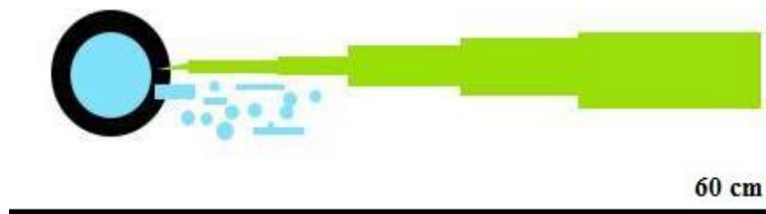
Figure 31. Depiction of the modelled environment. A root is penetrating a water pipe, causing leakage in a randomly distributed arrangement which has not homogenized.
