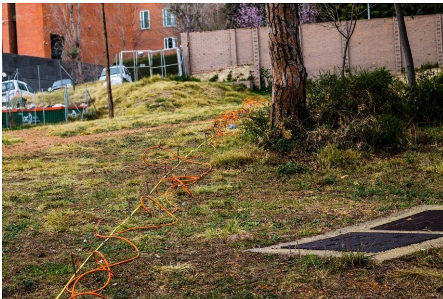
Figure 2. Commercial resistivity equipment (profile with electrodes) with 0.5 m spacing between electrodes.
