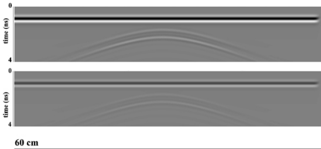
Figure 35. GPR response of a root of permittivity 12 (top) versus 8 (bottom) in an asphalt of permittivity 6.
