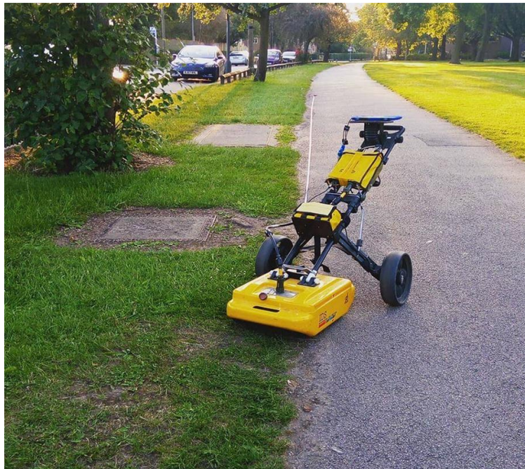
Figure 4. Typical GPR setup, prepared for measurement around UoB campus.
