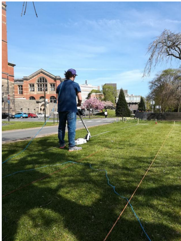
Figure 48. Typical soil survey using the 1.5 GHz Utsi antenna. Ropes and rulers were used to mark the survey area and ensure profile data acquisition on the right trajectory.
