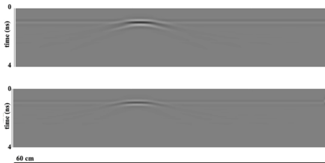
Figure 38. GPR response of a bump deformation with root (above) versus no root (below).
