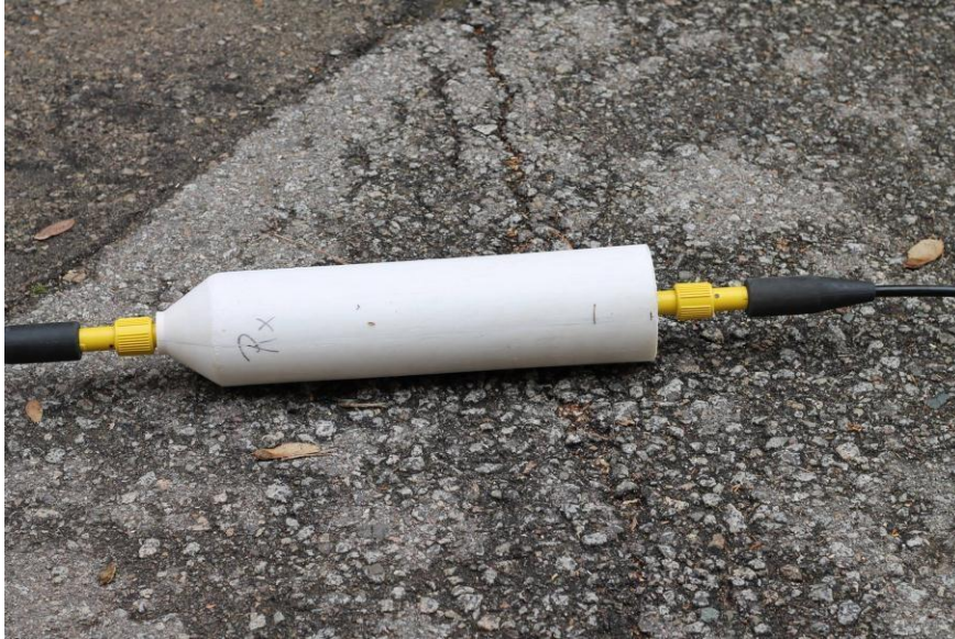
Figure 5. The Geometrics Ohmmapper, probably the most common capacitively-coupled resistivity meter in use at the moment, does not offer sufficient resolution to study tree roots effectively
