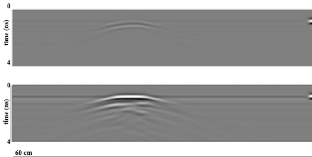
Figure 41. Comparison of the same system of cracks, air-filled (top) versus water-filled cracks (bottom).
