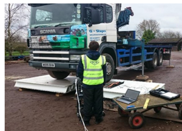
Fig 1. Field testing of deck panel using truck on outriggers
