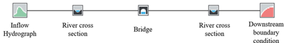
Fig. 6. Schematic showing a simplified setup with an inflow hydrograph, a river cross section, followed by a bridge, another river cross section and finally a downstream boundary condition.
