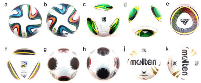
Figure 2 | Soccer balls used for the test and their panel orientations. (a, b) Adidas Brazuca: small dimple and six panels, (c, d) Adidas Cafusa: small grip texture and 32 modified panels, (e, f) Adidas Jabulani: small ridges or protrusions and eight panels, (g, h) Adidas Teamgeist 2: small protuberances and 14 panels; (i, j) Molten Vantaggio (conventional soccer ball): smooth surface and 32 pentagonal and hexagonal panels. (Photo by S.H.).
