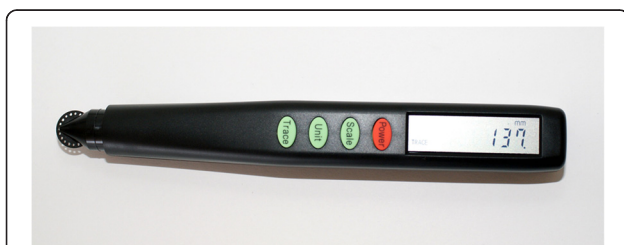
Figure 3 Example photo of the curvimeter for measuring extended total distances.
