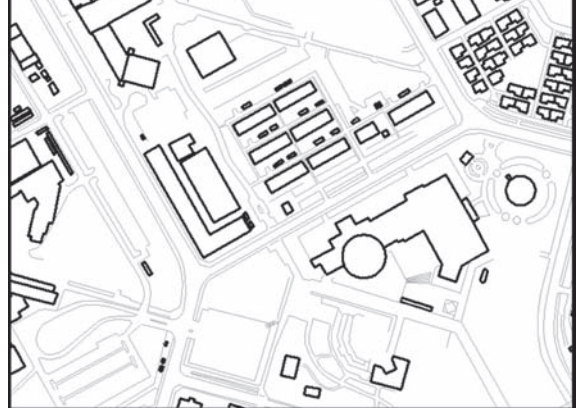
Fig. 3 Spatial adjustment performing between 2m above shaded Digital Height Model and building footprints
