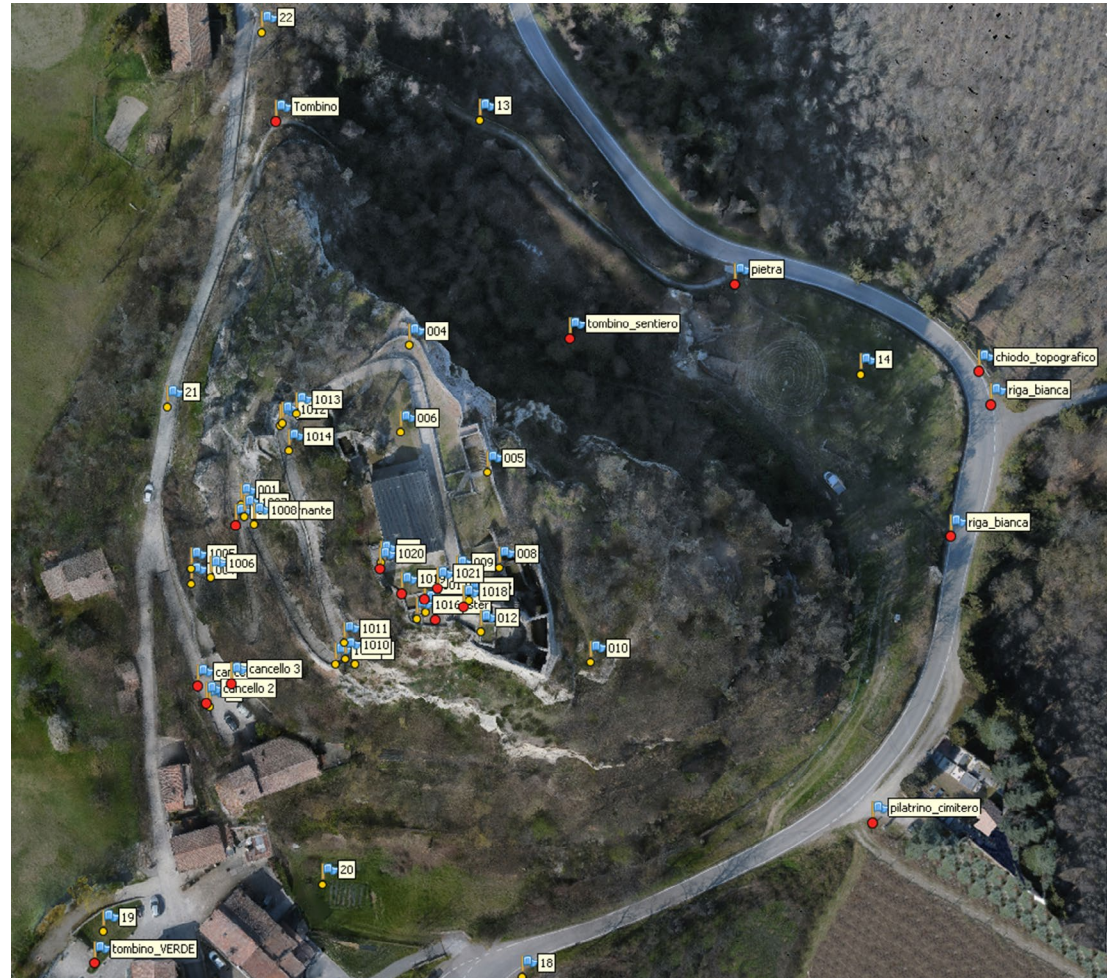
Fig. 8 - View from above with all artificial and natural points used in photogrammetric blocks.
