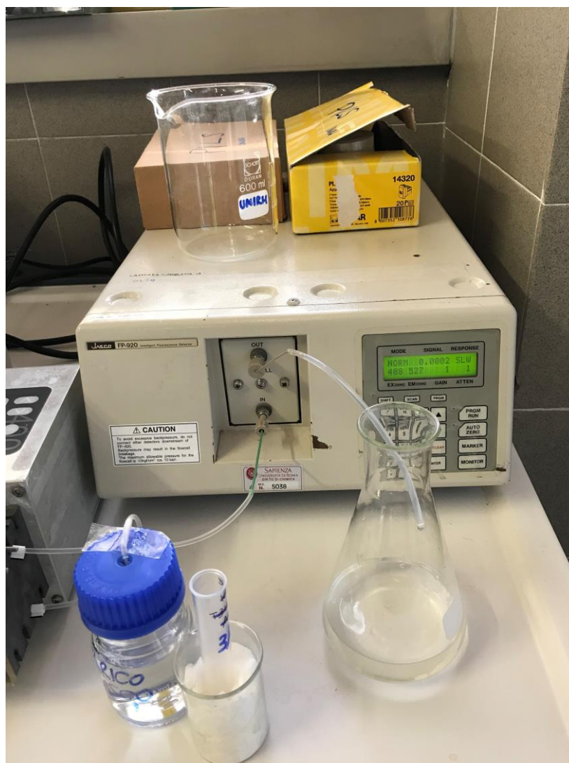
Figure 18. Fluorescence detector used for OP^{DCFH} measurements.
