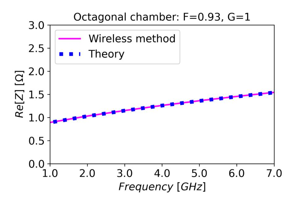
• Almost perfect agreement between the two curves suggesting -> the proposed simulation approach is a suitable and accurate method to compute the beam coupling impedance of arbitrary shaped chambers.
