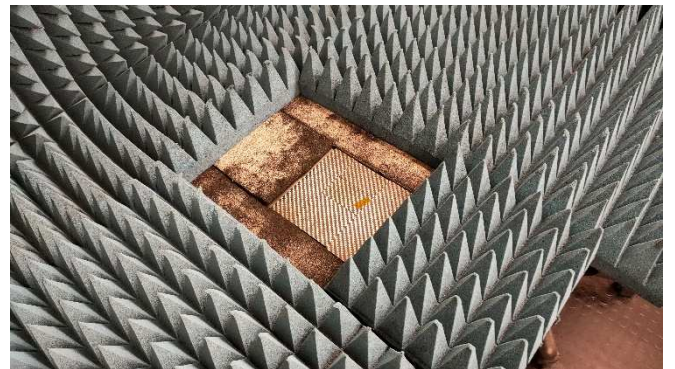
Fig. 9. The exposed sample surrounded by the anechoic panels
