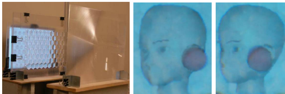
Figure 2: Prototype of coarse integral volumetric imaging (left) and the images observed from two different viewpoints with the prototype system (middle and right).
