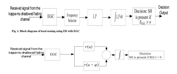
Fig. 2: Block diagram of local sensing using CD with EGC
