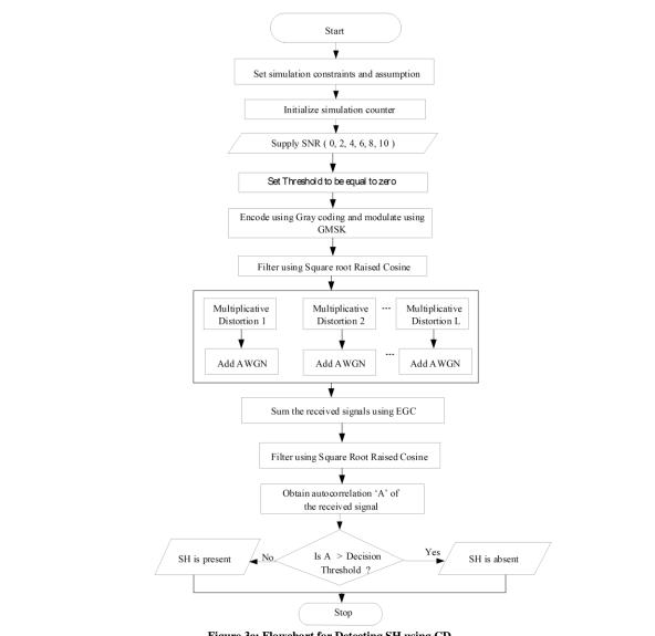
Figure 3c: Flowchart for Detecting SH using CD
