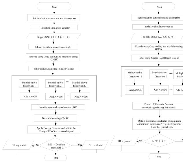
Figure 3a: Flowchart for Detecting SH using ED
