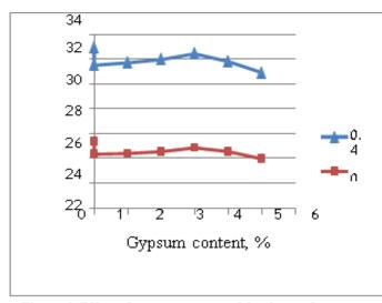
Figure 6: Effect of sugar-gypsum combination on the strength of concrete for various W/C ratio
