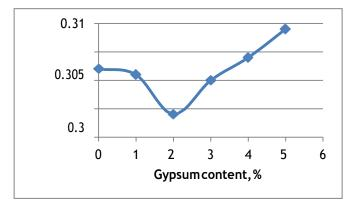
Figure 2: Effect of gypsum on the normal consistency of 0.02% sugar cement paste
