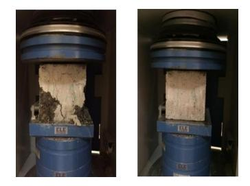
Figure 1: Cube test by compression testing machine
