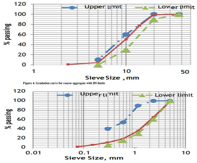
Figure 5. Gradation curve for the fine aggregate using wash sieving.
