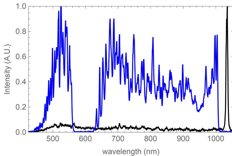
**Figure 2.** White-light continuum spectrum before (black) and after (blue) spectral filtering. The vertical scale is normalized separately for each measurement.
