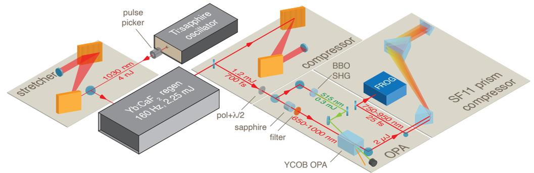
**Figure 1.** Schematic of the sub-picosecond pumped OPA experimental setup. pol+ $\lambda/2$ : half-wave plate and polarizer set; sapphire: supercontinuum generation stage; BBO SHG: second-harmonic generation stage; YCOB OPA: nonlinear amplification crystal; FROG: frequency-resolved optical gating diagnostic.
