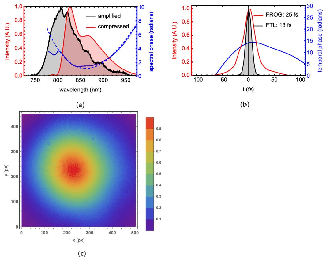
**Figure 3.** Compressed pulse FROG retrieval: (a) retrieved spectral intensity, phase and quadratic phase fit (red, solid blue and dashed blue, respectively), and spectrum measured at compressor input (black); (b) retrieved temporal intensity and phase (red and blue, respectively), and corresponding Fourier Transform limit duration (black); (c) Compressed beam spatial profile.
