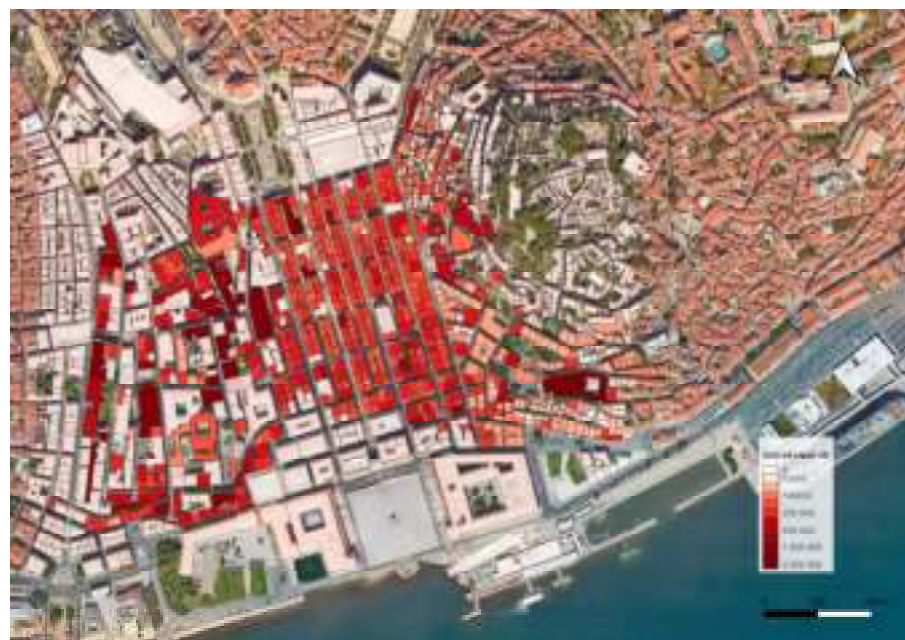
Figure 14. Cost of repair of Lisbon downtown (€).
