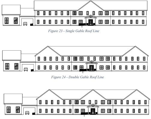
Figure 25 - Triple Gable Roof Line
