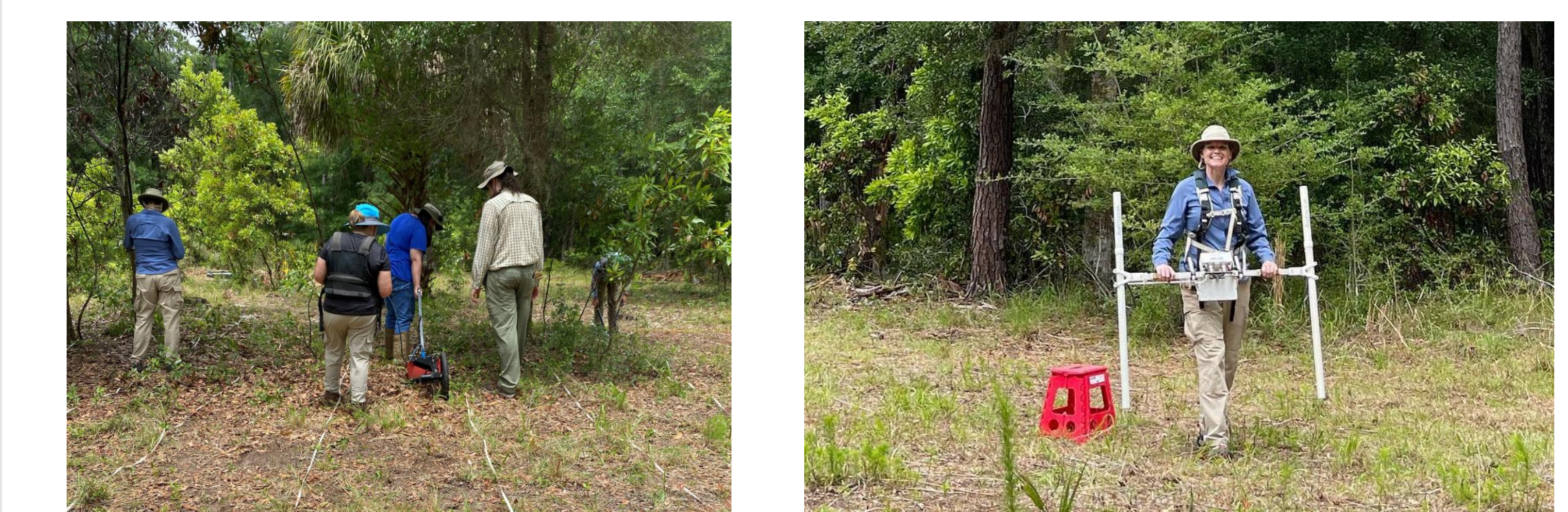
Ground penetrating radar with a 400 MHz antenna
