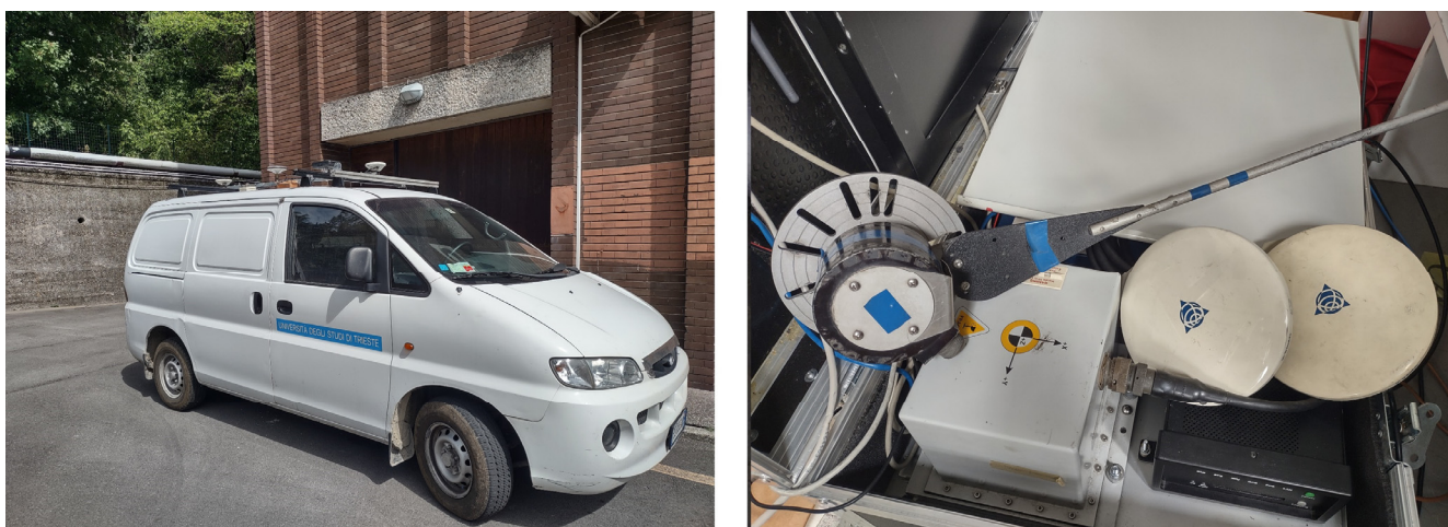
Figure 5. The MMS of the GeoSNav Lab, University of Trieste, and the Applanix Corporation POS/LV© system components mounted on board the vehicle. MMS data were used to create the reference trajectory.
