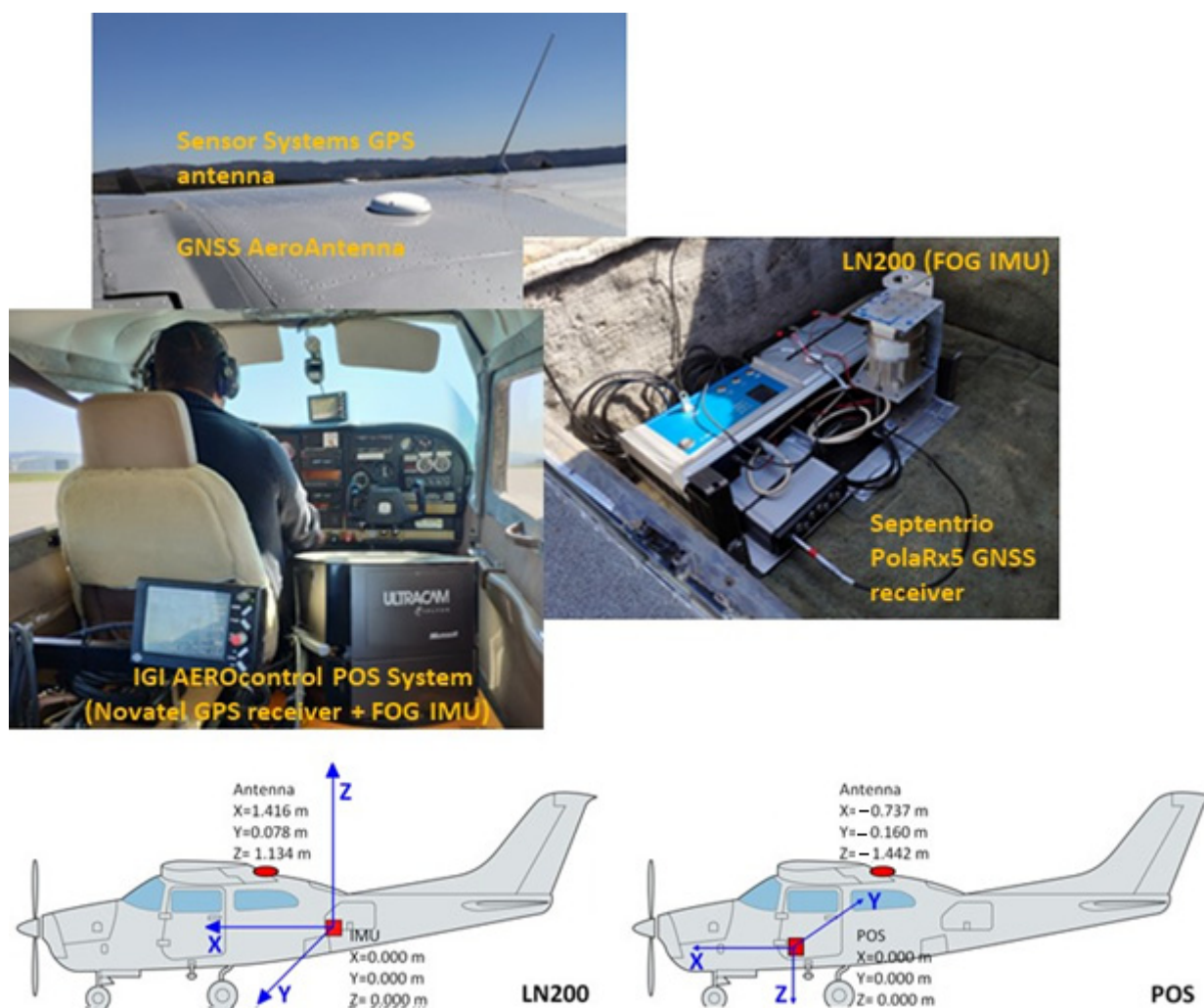
Figure 3. Equipment used in the aerial data-collection campaigns. Left: Septentrio receiver, LN200 IMU and data logger; Middle: POS system; Right: AeroAntenna (foreground) and Sensor Systems antenna (background) fixed on the aircraft.
