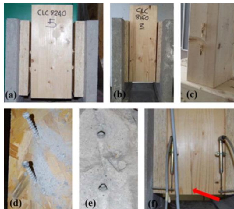
Figure 7. Failure mechanisms for the examined TCC connections in push-out experimental tests: examples of (a–c) recurring mechanisms or (d–f) infrequent failure modes. Red arrow: failure.
