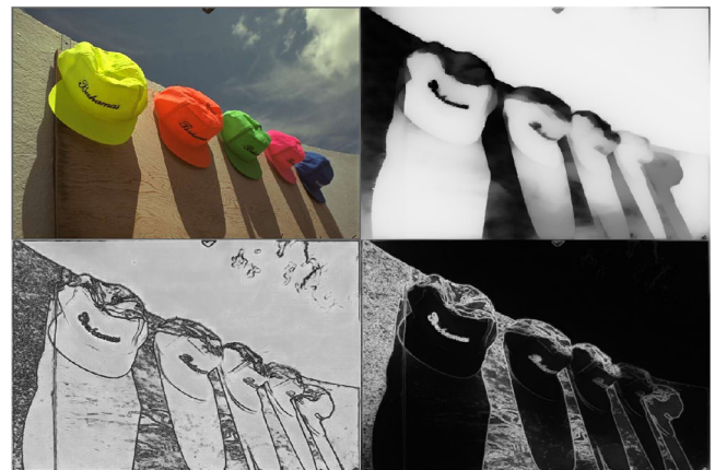
FIGURE 19 JPEG image and corresponding maps. Top-left is “Caps” after JPEG compression with Q = 60 , top-right is the blur map for the image, bottom-left gives the artifact map while bottom-right gives our combined map used for artifact-reduced enhancement
