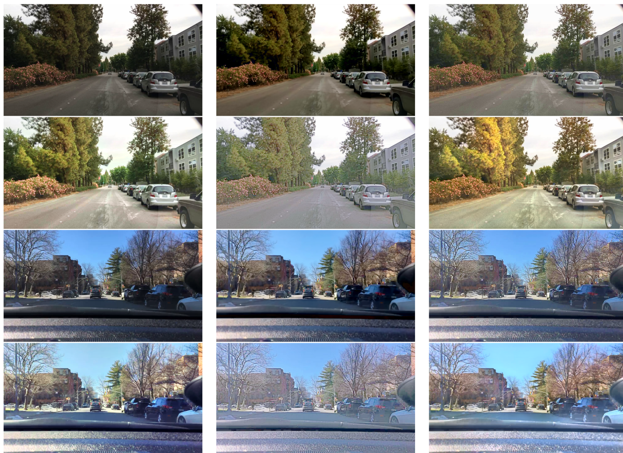
FIGURE 21 Enhancement results using different low light enhancement techniques on Berkeley Driving Dataset Images. Top row shows Original, MBLLEN, NLBM from the left while bottom row shows DUPE, ZDCE, EGAN from the left
