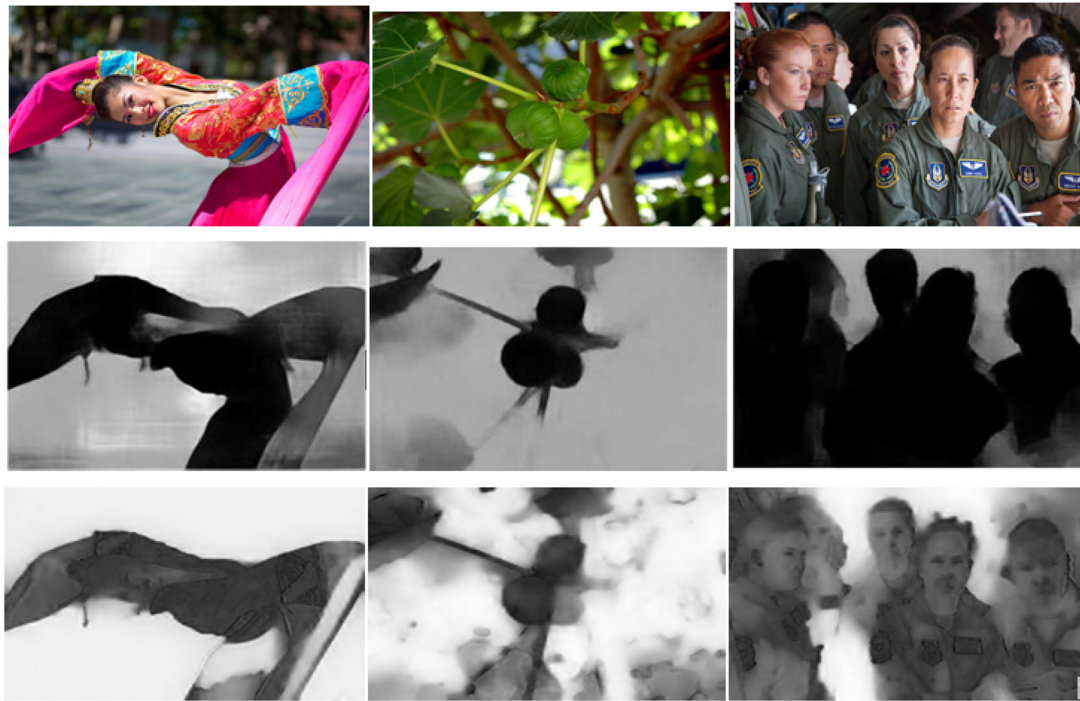
FIGURE 12 Blur maps derived with the method in [30] (middle row), and our method (bottom row) using sample images from CUHK dataset
