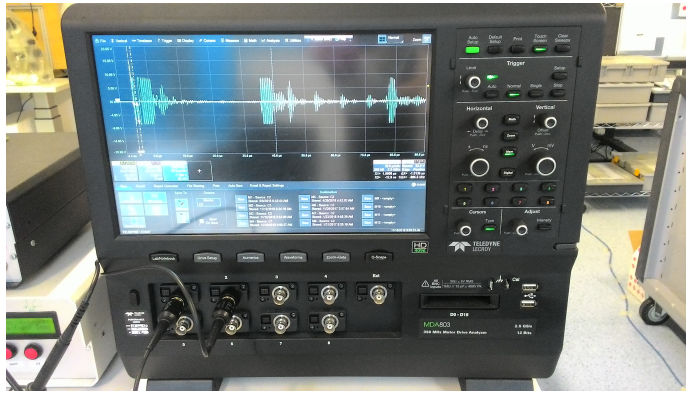
Figure 4.8: Teledyne LeCroy MDA803 digital scope, 8 channel, sampling rate 2.5GS/s.
