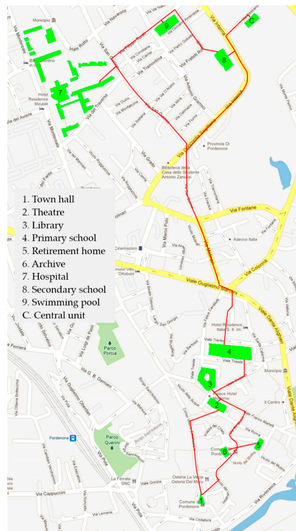
Figure 3. Possible connections for the DHCN pipelines.
