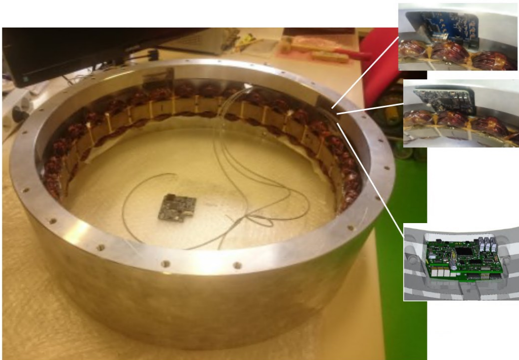
Fig. 38 Machine stator frame and compartments for AC/DC power electronics board installation.
