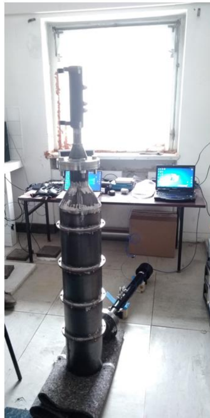
Figure A3-VII: Model-scale scrubber with tower packing.
