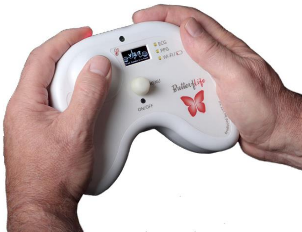
Figure 1. The ButterfLife device. In order to perform a test, the device needs to be held between both hands for 90 s with palms placed on the lateral electrocardiography sensors and fingers placed on the photoplethysmography sensors.
