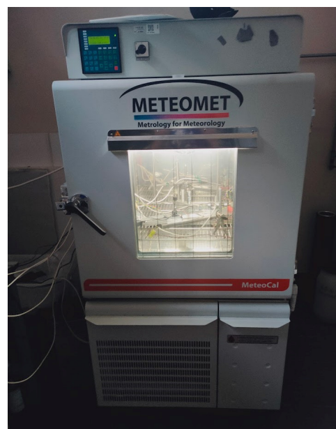
Figure 1. Climatic chamber Kambic MeteoCal KK-105 in operation at INRiM and used to test RS92 and RS41 under various temperature and humidity conditions and ambient pressure. The chamber simultaneously and independently controls temperature (range -40\text{ °C} < T < 180\text{ °C} ) and relative humidity (range 10\% < RH < 98\% in the temperature range 10\text{ °C} < T < 95\text{ °C} ).
