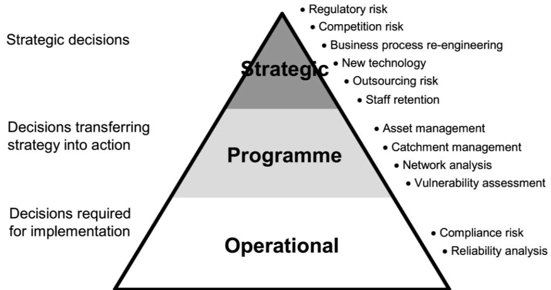
Figure 2.5: Conceptual illustration of the risk hierarchy for water services providers, comprising risks on strategic, programme, and operational levels (reproduced from MacGillivray et al., 2006).
