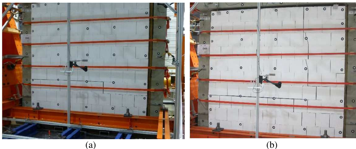
Figure 56 (a) Appearance of the first crack in the wall (Marinković 2018); (b) Cracks in the wall at the end of Phase 4 (Marinković 2018)
