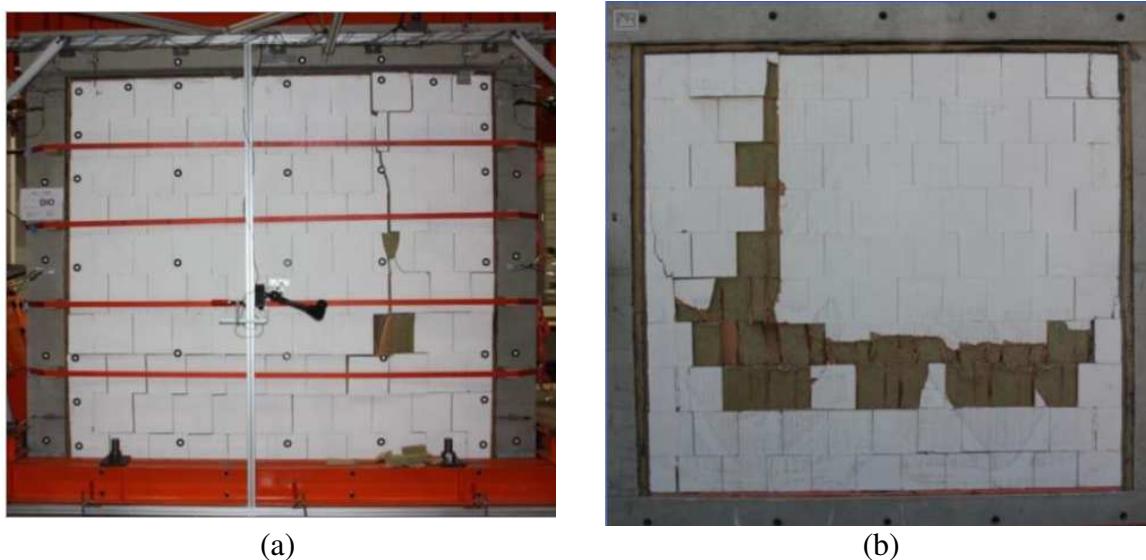
Figure 57 (a) Damage at the front side at the end of DIO test (Marinković 2018); (b) Damage at the back side at the end of DIO test (Marinković 2018)
