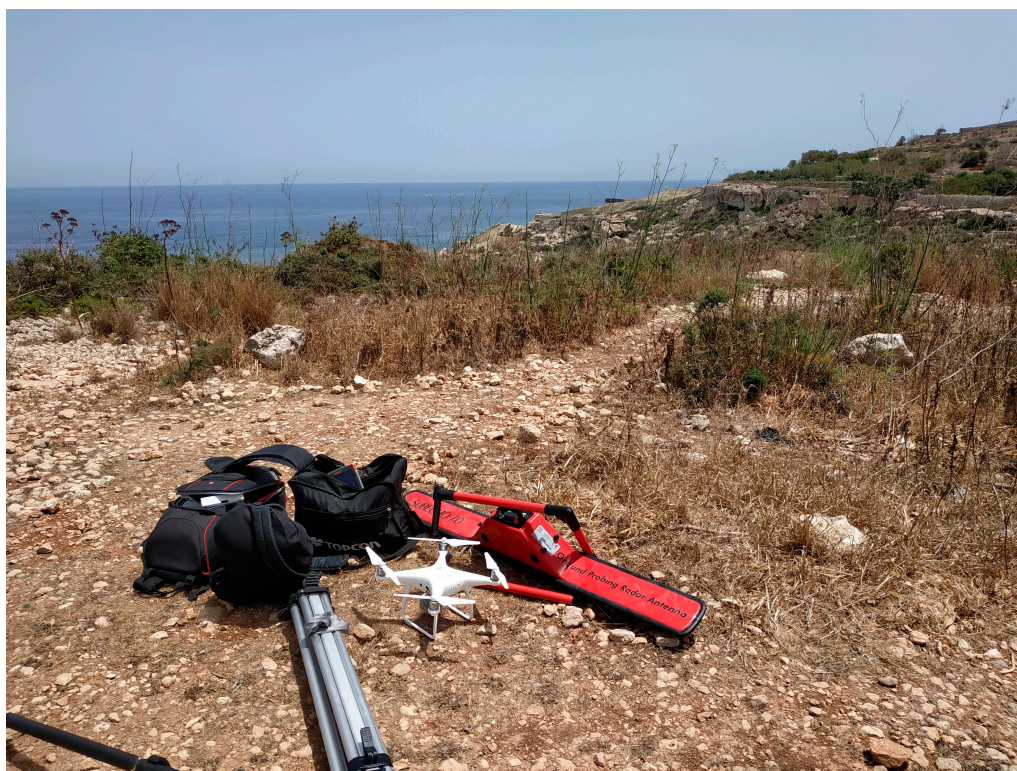
Figure 3. Photo acquired during the georadar survey. The photo shows the tripod and rod of the Differential GNSS, the Phantom 4 Pro UAV used for photogrammetric survey and the Cobra Subecho-70 georadar.
