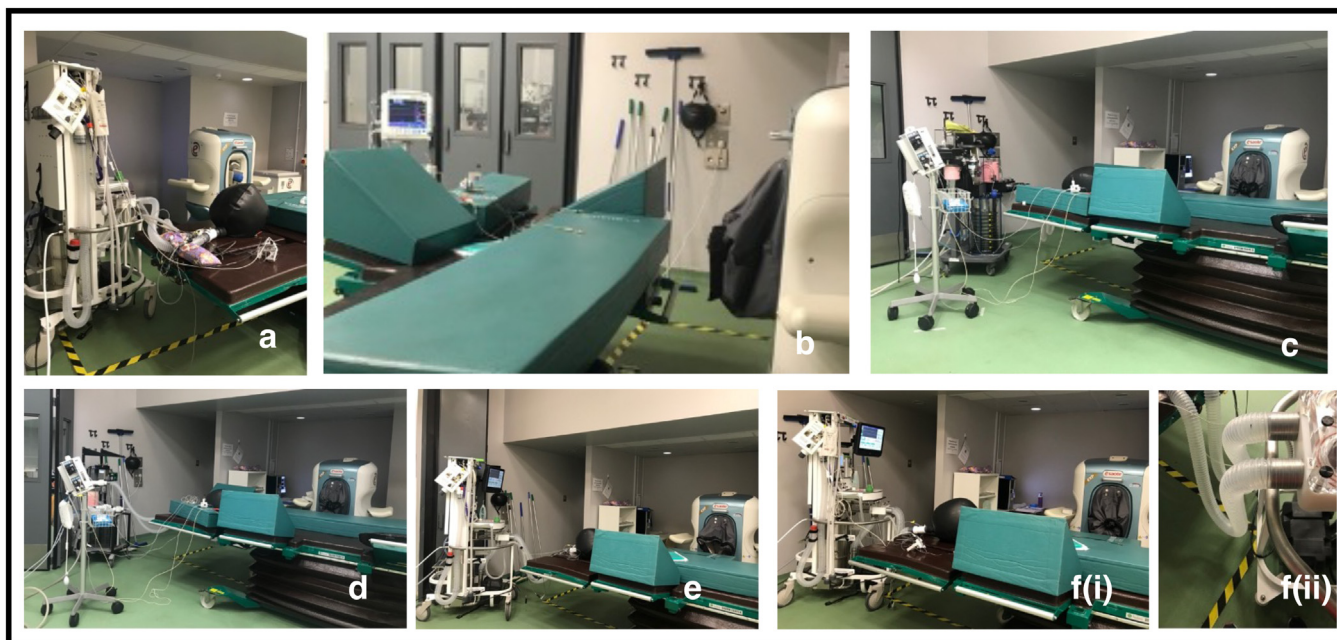
Fig. 3. Set up of 6 of the seven conditions tested (the negative control is not displayed). (A) Positive control: MRI RF shields removed and Tafonius positioned within the controlled area; (B) Standard monitoring only: Datex S5 monitor on, monitoring equipment, and equine surgery table positioned as in normal clinical cases; (C) Mallard anaesthesia machine positioned as for standard clinical cases; (D) Bird anaesthesia ventilator positioned as for standard clinical cases; (E) Tafonius with integrated monitor on placed as for standard clinical cases; (F) Tafonius in close proximity (i), with detail of the front frame on the boundaries of the controlled area (ii).
