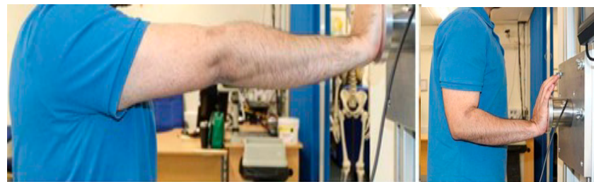
Figure 6. Hand forces with the shoulder joint in 90 deg with the trunk (left) and hand pushing forces with the elbow joint in 90 deg (right).
