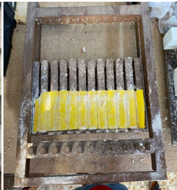
Photo (16) Soap-cutting machine instead of wire.
