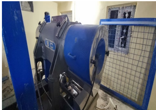
Photo (12) A machine for separating oil from the core and water.
