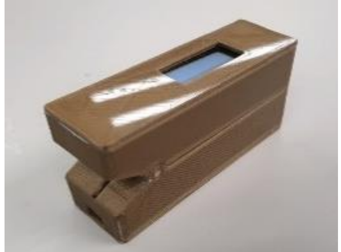
Fig. 1. Developed BP, HR and SpO 2 monitor, enclosed in a 3D case with a 0.91" OLED display to be worn on the finger of the user
