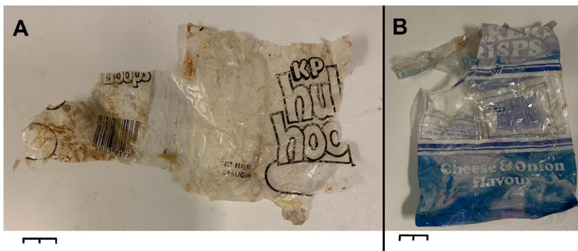
Figure 3.6. Two crisp packets, both over 30 years old. A) A KP Hula Hoops packet for which the age could be determined by a best before date printed on the front (09 Aug 86); B) A Walkers crisp packet assumed to be 30 years old based on similar reports (Tracey, 2018) and changes in the Walkers logo (Logopedia, 2020). Scale bars = 2 cm.
