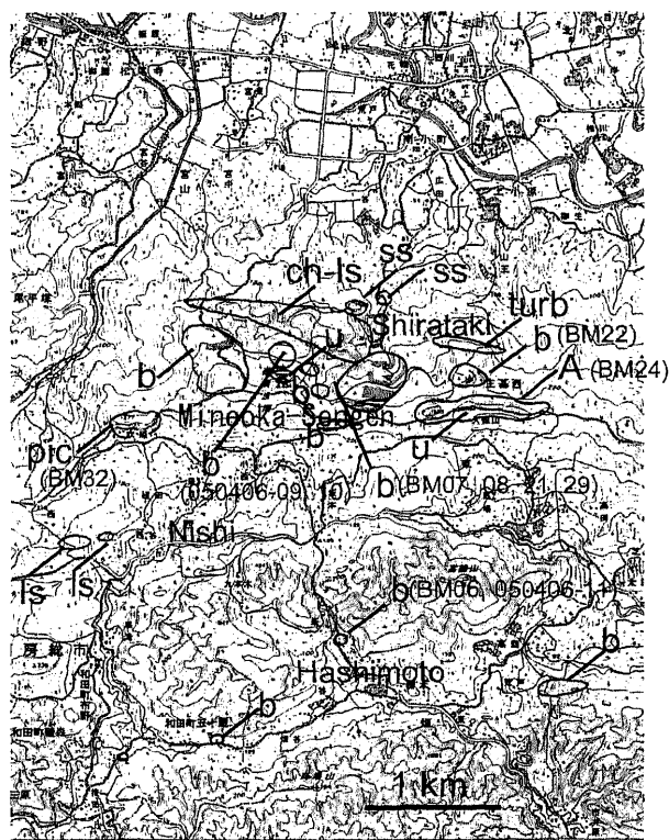
Fig. 12 Knocker distribution map in the Mineoka-Sengen area with sample number. Abbreviation of rock type other than in Figs. 3 and 11 is as follows. ch-ls: alternation of chert and limestone, ls: limestone, pic: picrite, ss: sandstone, turb: turbidite (part of the Shimanto Supergroup).
