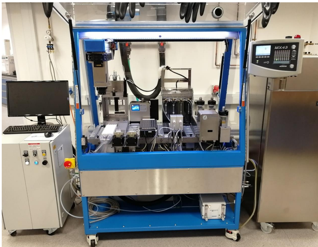
Figure 13: The University of Bristol Chemspeed Automation Platform, including Huber cryostat on the right.
