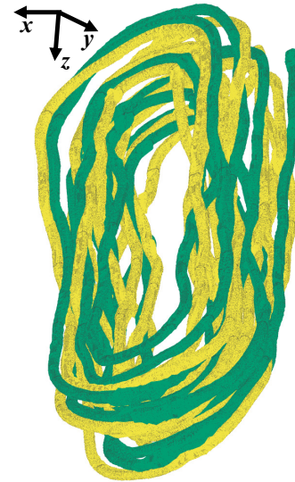
Fig. 8. Evidence of twisted strand transposition between Strands 4 and 5
