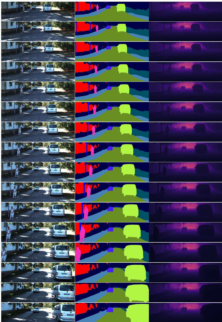
Fig. A4: Prediction visualizations on SemKITTI-DVPS. From left to right: input images, temporally consistent panoptic segmentation (TCPS), and depth predictions. Color change of the same instance of TCPS indicates an id switch.
