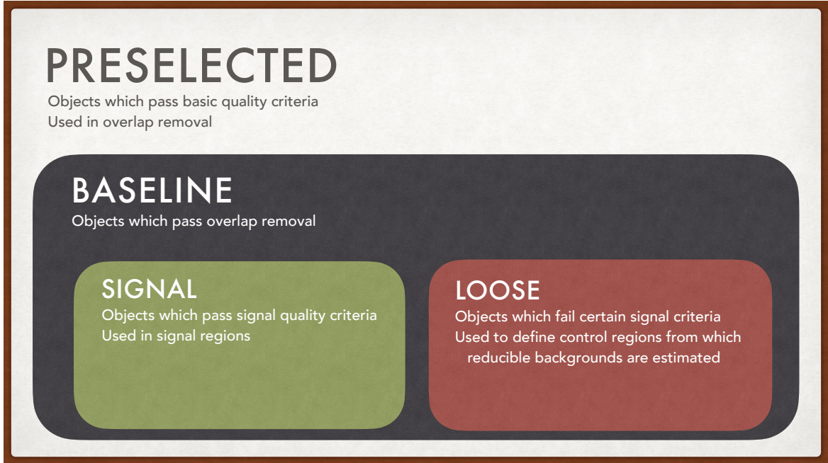
Figure 5.5: Diagram showing the relationships between and uses of preselected, baseline, signal, and loose object selections
