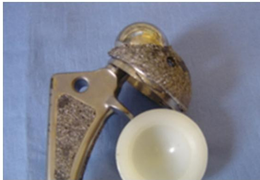
Figure 9.3 – Femoral head and cup showing an area of severe wear
