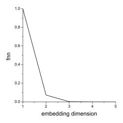
Fig. 3. Determination of the minimal required embedding dimension. The fraction of false nearest neighbours (fnn) drops convincingly to zero at m = 3.
