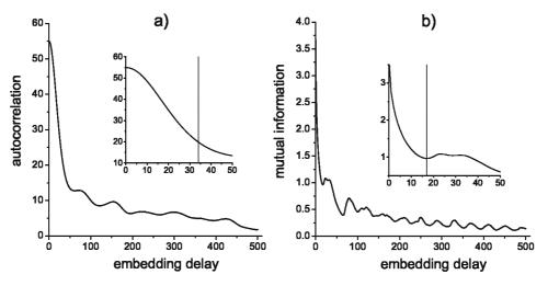
Fig. 2. Determination of the proper embedding delay. a) The autocorrelation decays to 1/e at  $\tau = 34$ . b) The mutual information has the first minimum at  $\tau = 17$ .
