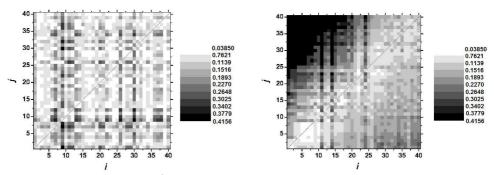
Fig. 4. Stationarity test. a) Cross-prediction errors obtained for the original time series. b) Cross-prediction errors obtained for the time series calculated with variable parameters during recording.
